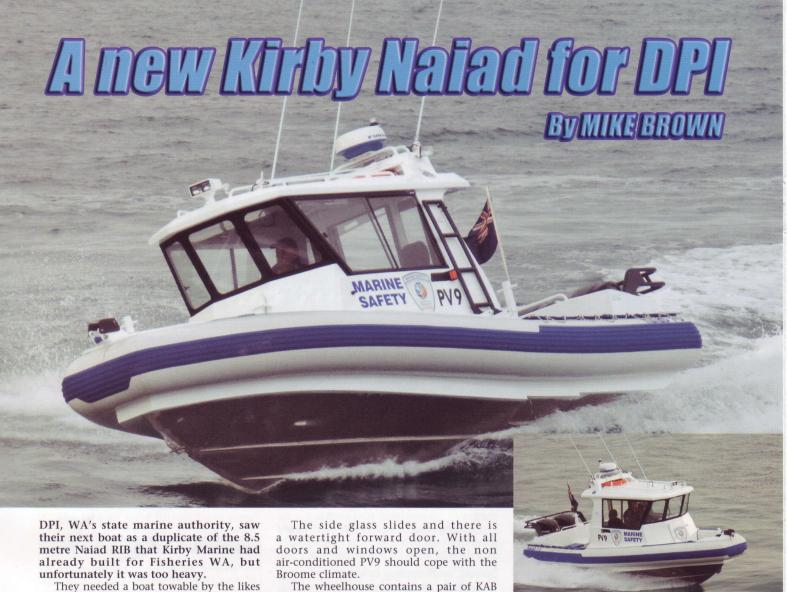
They needed a boat towable by the likes of a Land Cruiser, which meant an all-up weight under 3.5 tonnes. So they asked for as near a duplicate as possible within the critical weight. This evolved into a 7.3 metre Naiad, PV9.
